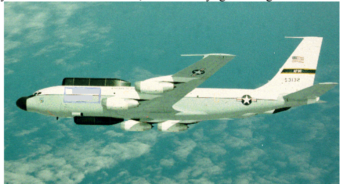
Fig. 2. Airborne Radar Platform (BCPO KC-135) with VHF Antennas Mounted on the Cargo Bay Door
